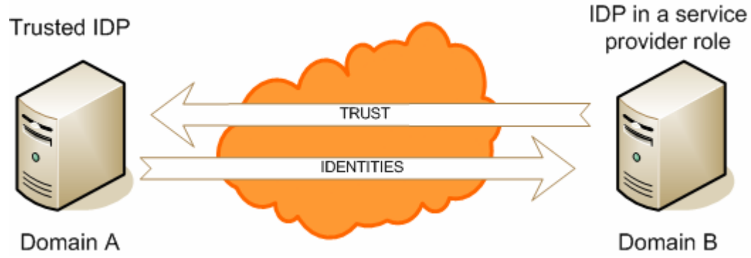
Figure 2 Domain B trusts Domain A, and the Domain B identity provider functions in a Service Provider role
